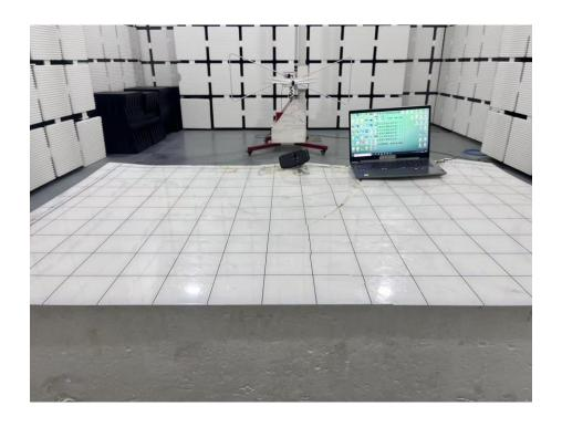
Set-up for Radiated Spurious Emission, Above 1GHz
