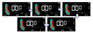
(4) 5-grid display of battery level: when the battery is full, the 5-grid lights are all on, and the battery flashes when the battery is under-voltage, indicating that it needs to be charged immediately. As shown below:
