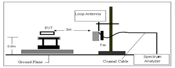
(B) Radiated Emission Test-Up Frequency 30MHz~1GHz
