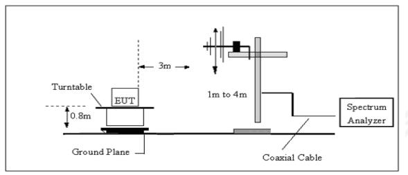
(C) Radiated Emission Test-Up Frequency Above 1GHz
