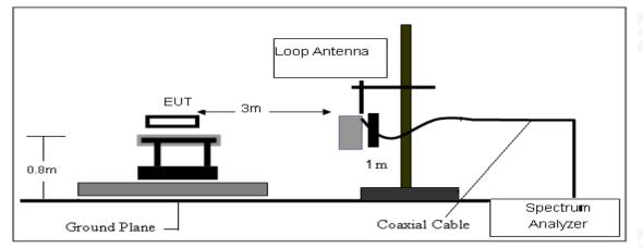
(B) Radiated Emission Test-Up Frequency 30MHz~1GHz
