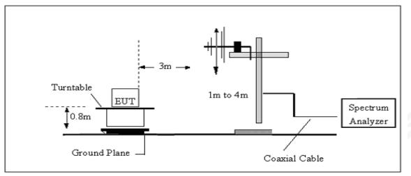
(C) Radiated Emission Test-Up Frequency Above 1GHz
