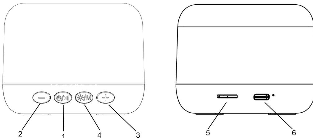
1: Switch On/Off button. Long press of 3 second for Switch on/off. Short press for Pause/Play function.
