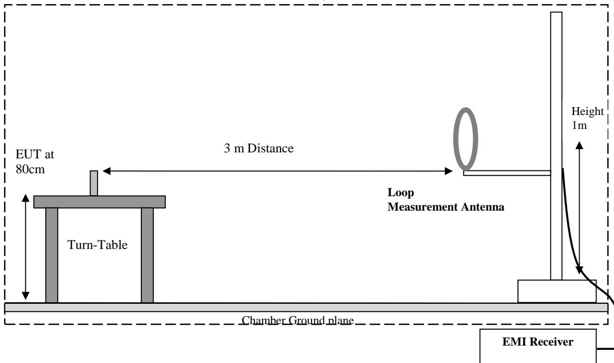
Radiated Emissions Test Setup 30MHz-1GHz Measurements
