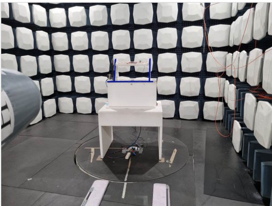
Photograph 2: EUT test setup in the fully anechoic chamber, overview_EUT elevation 0°
