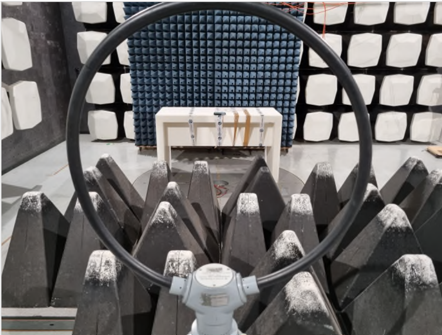
Photograph 6: EUT test setup in the semi anechoic chamber with floor absorber for H-Field measurement, overview_EUT elevation 0°
