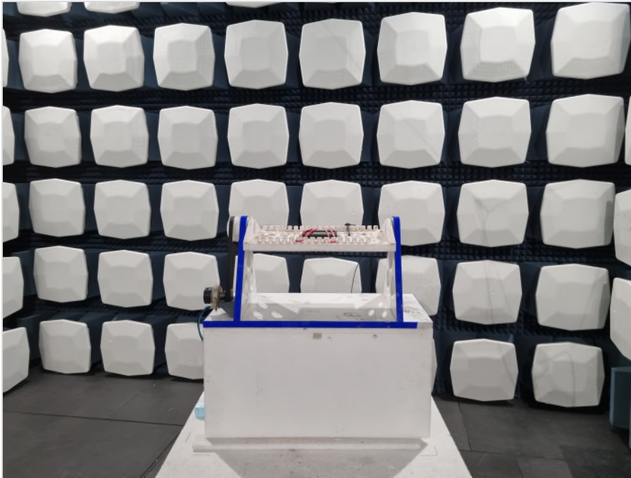
Photograph 1: EUT test setup in the fully anechoic chamber, close up view_EUT elevation 0°
