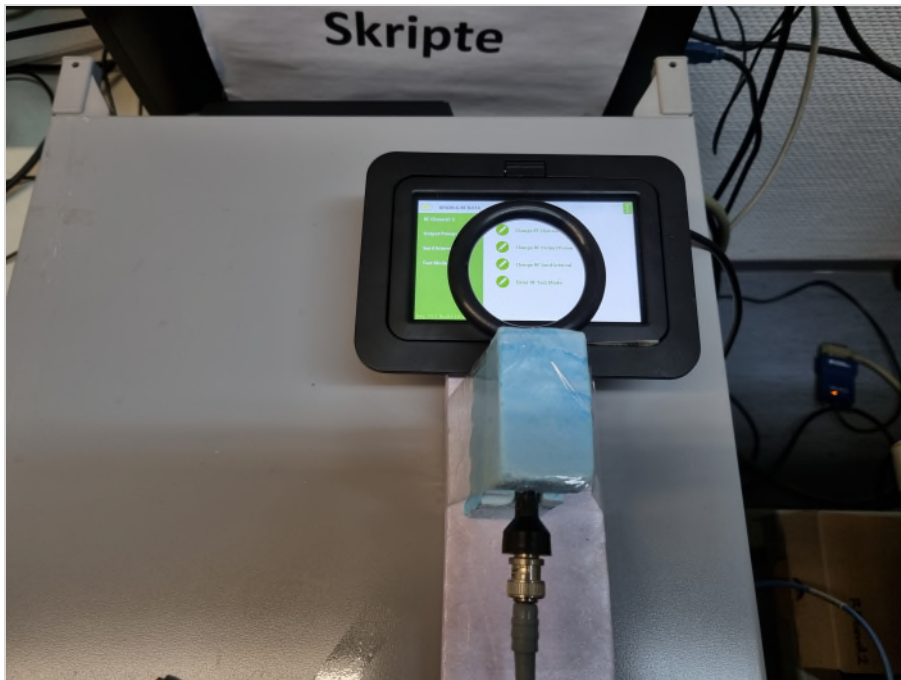
Photograph 11: EUT setup conducted measurement with near field probe, close up view
