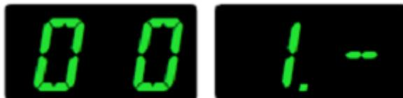
When you select the program you can choose the projector which wants to attribute the scene (from 1-9). Press button "B". The display of "PROJ." will indicate a blinking dot. Then select the number with the buttons "UP" or "DOWN."
