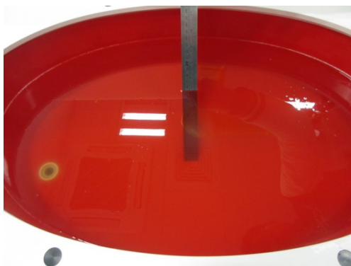
Liquid depth in the flat Phantom ( \geq 15\text{cm} depth) HSL(2450MHz)
