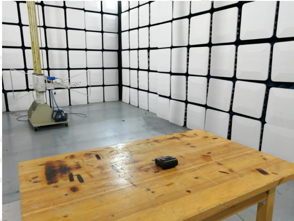
Photo of Radiation Emission Test
