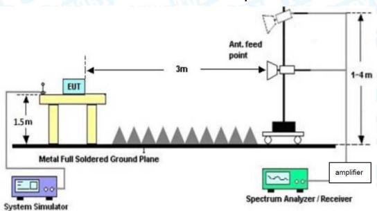
**Above 1GHz Test Setup**
