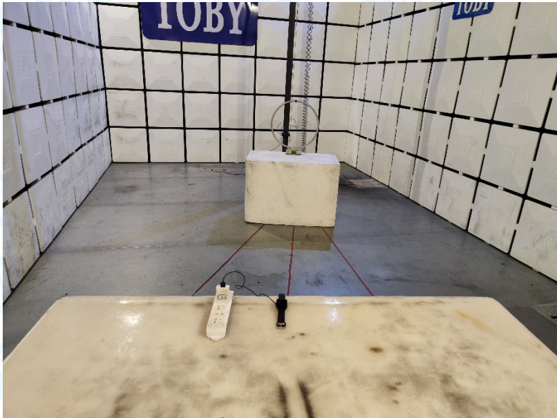
Photo of Setup for Radiated Emission (9KHz-30MHz)
