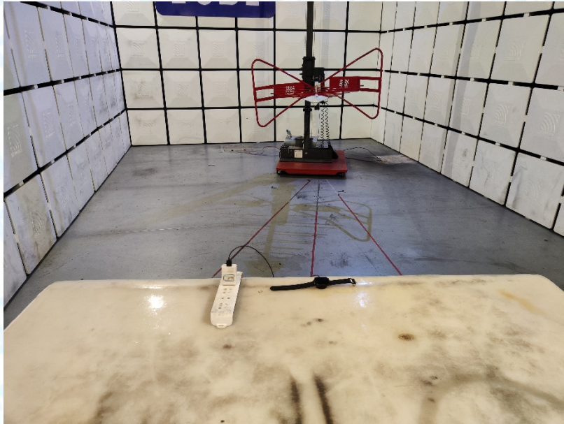
Photo of Setup for Radiated Emission (9KHz-30MHz)
