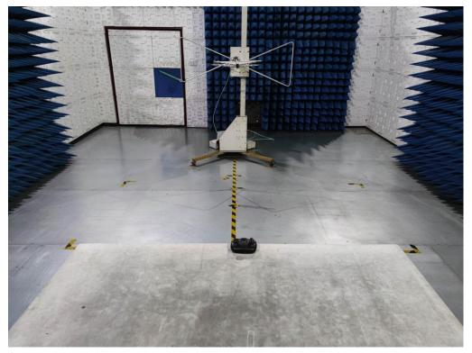
RADIATED EMISSION TEST SETUP ABOVE 1GHz
