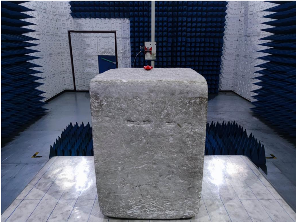
RADIATED EMISSION TEST SETUP ABOVE 1GHZ
