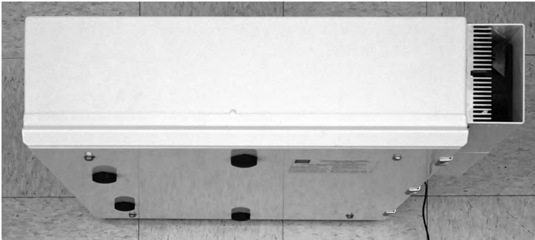
Fig. 14. Synthesizer-Transmitter Unit, top view. The twin-fan forced air flow heat exchanger unit is seen on the right side.
