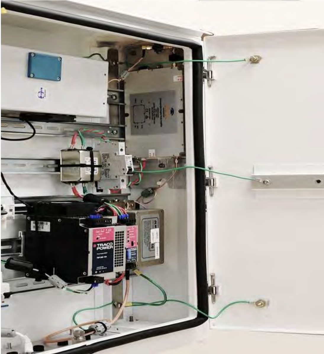
Figure 10. Synthesizer-Transmitter Unit, door open, slanted view. The power amplifier module (top) and the low-pass filter (bottom) are seen on the right inner wall.
