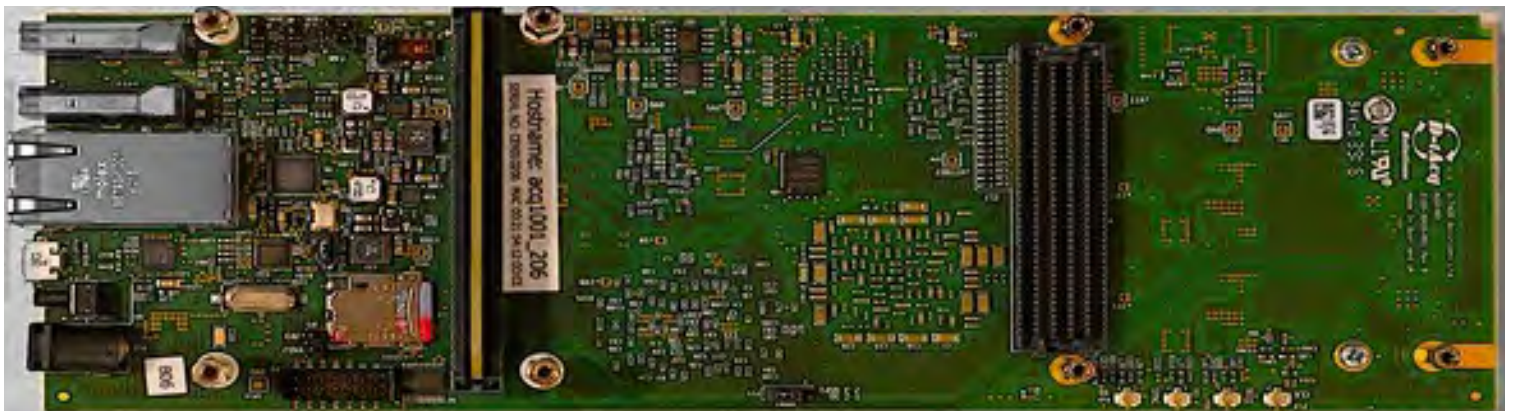
Figure 3c. Photo of the carrier board with FPGA (top face; bottom face not accessible).
