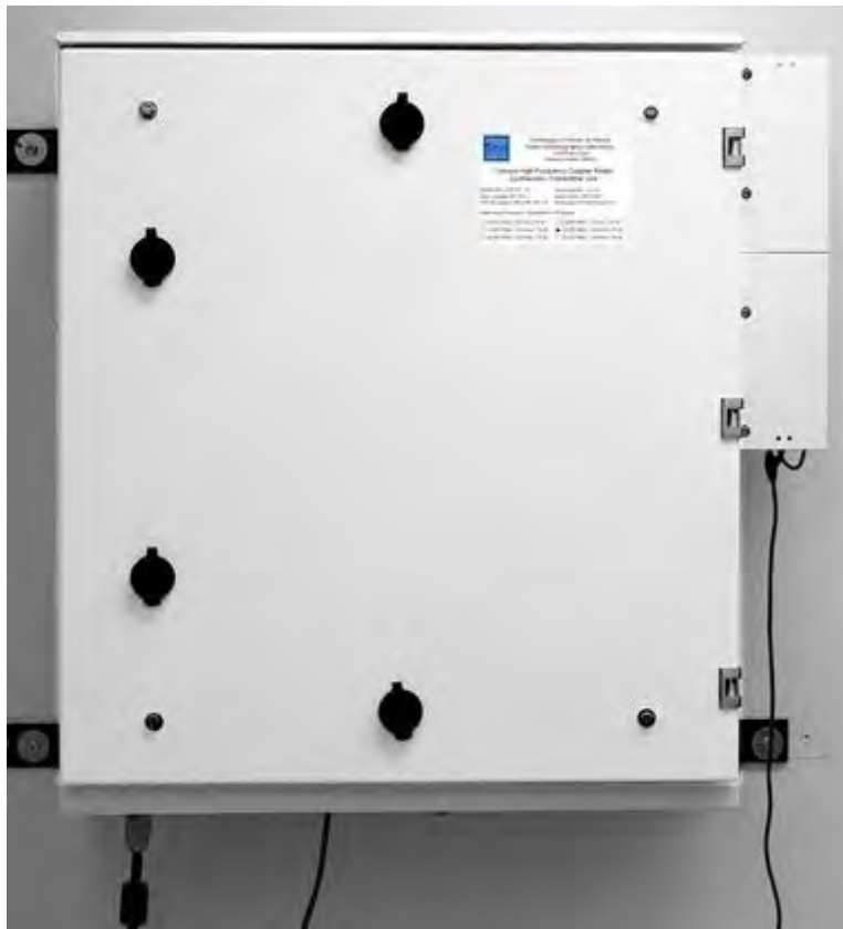
Figure 8. Above: Synthesizer-Transmitter Unit model MK3-PW-PA-TX, serial 3-003 (March 2022), door closed. Below: device identification label, affixed to the top right of the enclosure door. The factory-programmed operating frequency and output power are marked, here 16.150 MHz/30W.
