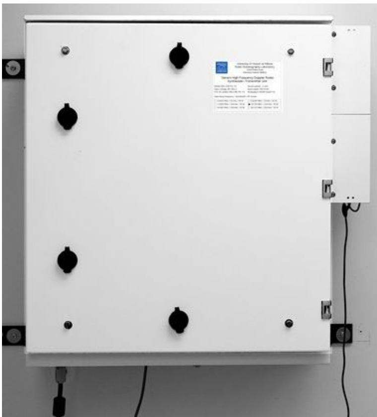
Figure 3. Above: Synthesizer-Transmitter Unit model MK3-PW-PA-TX, door closed. Below: device identification label, affixed to the top right of the enclosure door. The factory-programmed operating frequency and output power are marked, here 16.150 MHz/30W.
