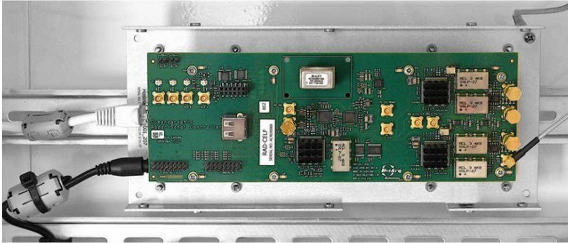
Figure 3. Upper rail enlarged from Figure 1 and 2, after removal of the aluminum lid and thermal bell, showing the Triple DDS Radar Controller board.
