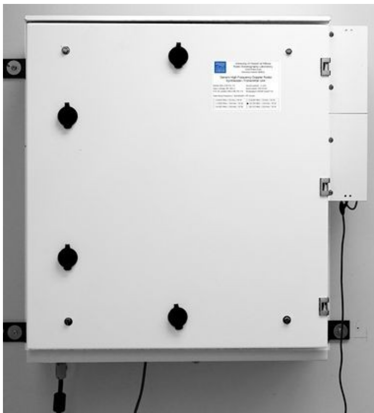
Figure 1. Above: High Frequency Doppler Radar Synthesizer-Transmitter Unit model MK3-PW-PA-TX, serial 3-003, door closed. Below: device identification label, affixed to the top right of the enclosure door. The factory-programmed operating frequency and output power are marked, here for example 16.150 MHz/30W.
