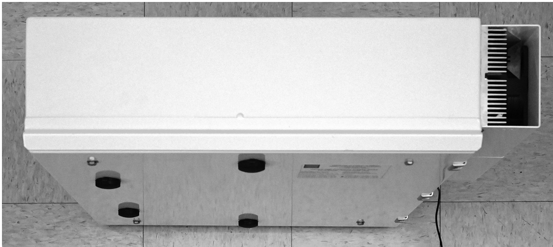
Fig. 4. Synthesizer-Transmitter Unit, top view. The twin-fan forced air flow heat exchanger unit is seen on the right side.
