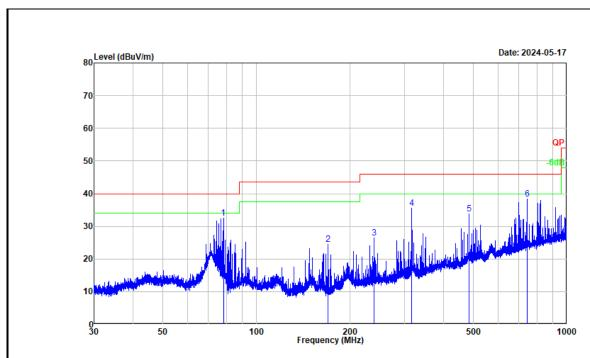
Project No. : RWAZ202300090 Test Mode : Transmitting Test Voltage : AC 120V/60Hz
