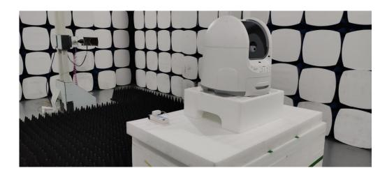
Note: the antenna of the EUT was located at height of 1.5 m above the floor
