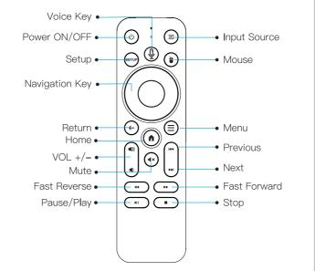
Paring method( Bluetooth mode connection) 1. Select [Settings] > [Bluetooth & Remotes] > [Add accessory]. 2. Press and hold the left & right direction buttons at the same time for 3-5 seconds until the red light flashes.
