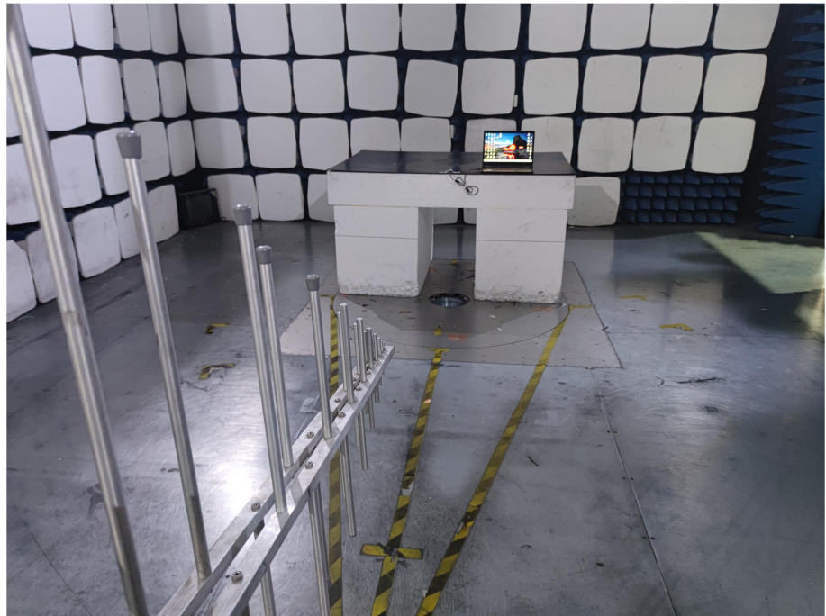
Radiation Emission Test Setup (30MHz to 1GHz)
