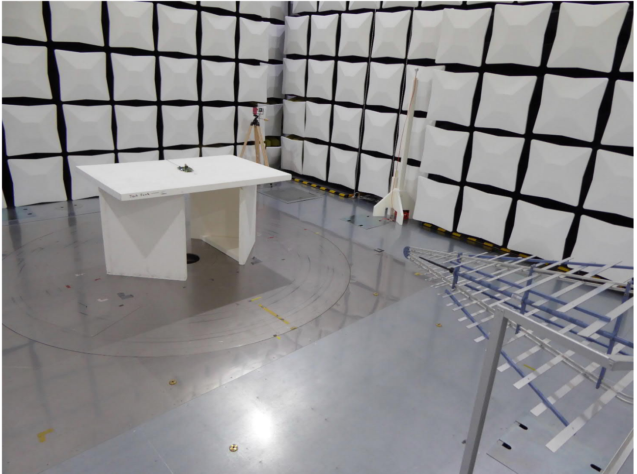
Test setup anechoic chamber (#44)
