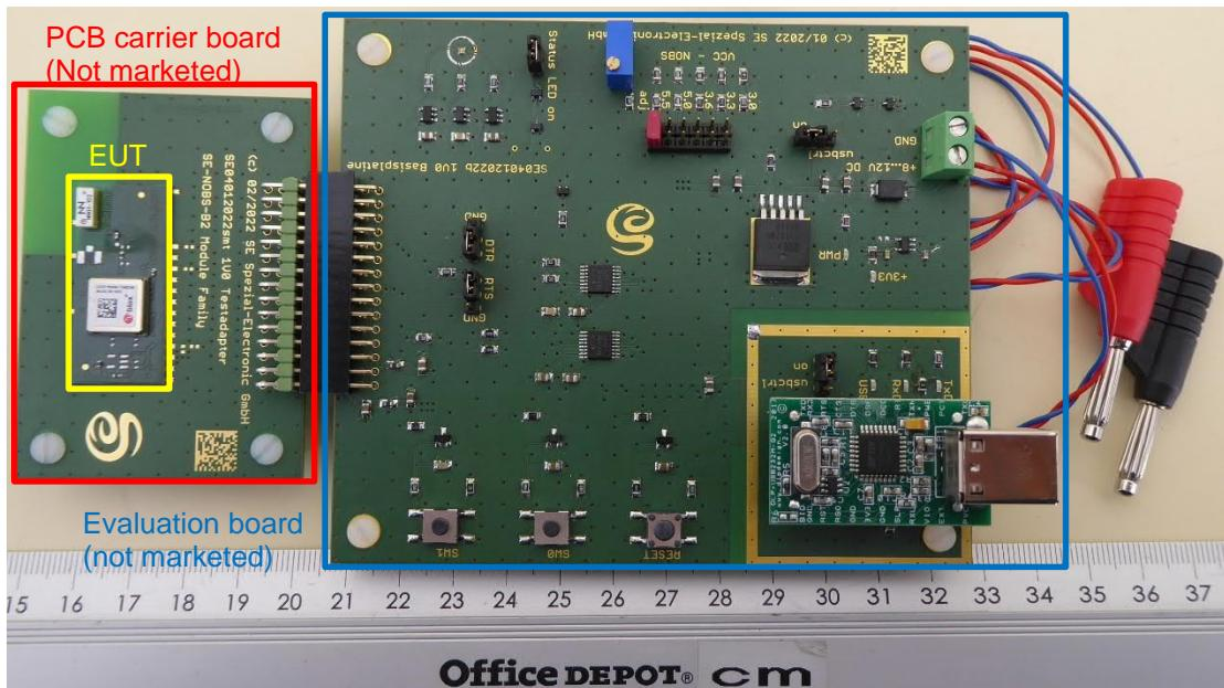
To start the test mode, two pins on the EUT PCB have to be shortened and the reset button on the evaluation board has to be pressed simultaneously. During the tests, a test laptop was connected to the EUT via USB to fiber-optic-converters. The test firmware was loaded to the EUT, using a command in the command prompt. The test commands were sent to the EUT via a terminal application. The test firmware and the test commands were provided by the applicant.
