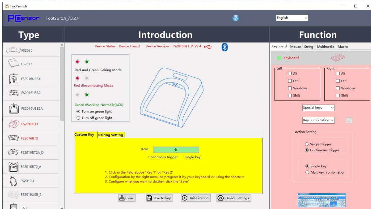
Clear button can delete the currently set key value, Save to key button used to save the current Settings, Initialization button used to restore the function to factory Settings, Device Settings used to set low power alarm function, When low power
