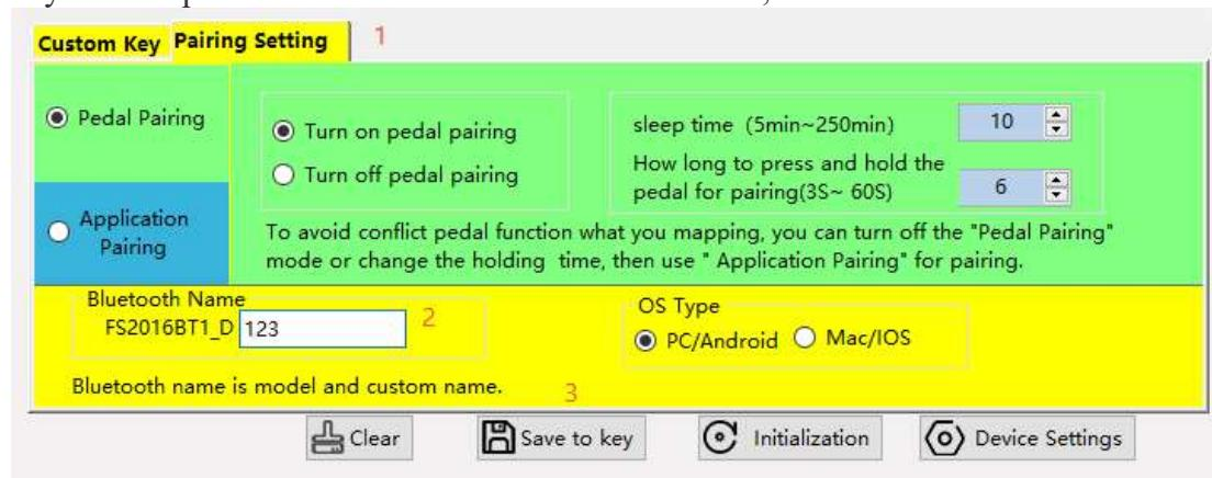
**Set the sleep time:** Click “Pairing Setting” to set the sleep time in the input box of sleep time. The sleep time indicates how long the device will enter the sleep state after no action (Pedal no action).
