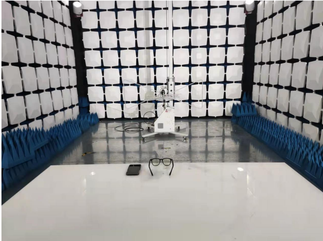
Above 1GHz for radiated emission test setup
