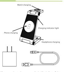
After connecting to the power supply, the blue indicator lights up, and automatically turns off after three seconds, and the charging board enters the standby state. 2. The mobile phone with wireless charging function is placed on the charging board, and the LED indicator lights up.
