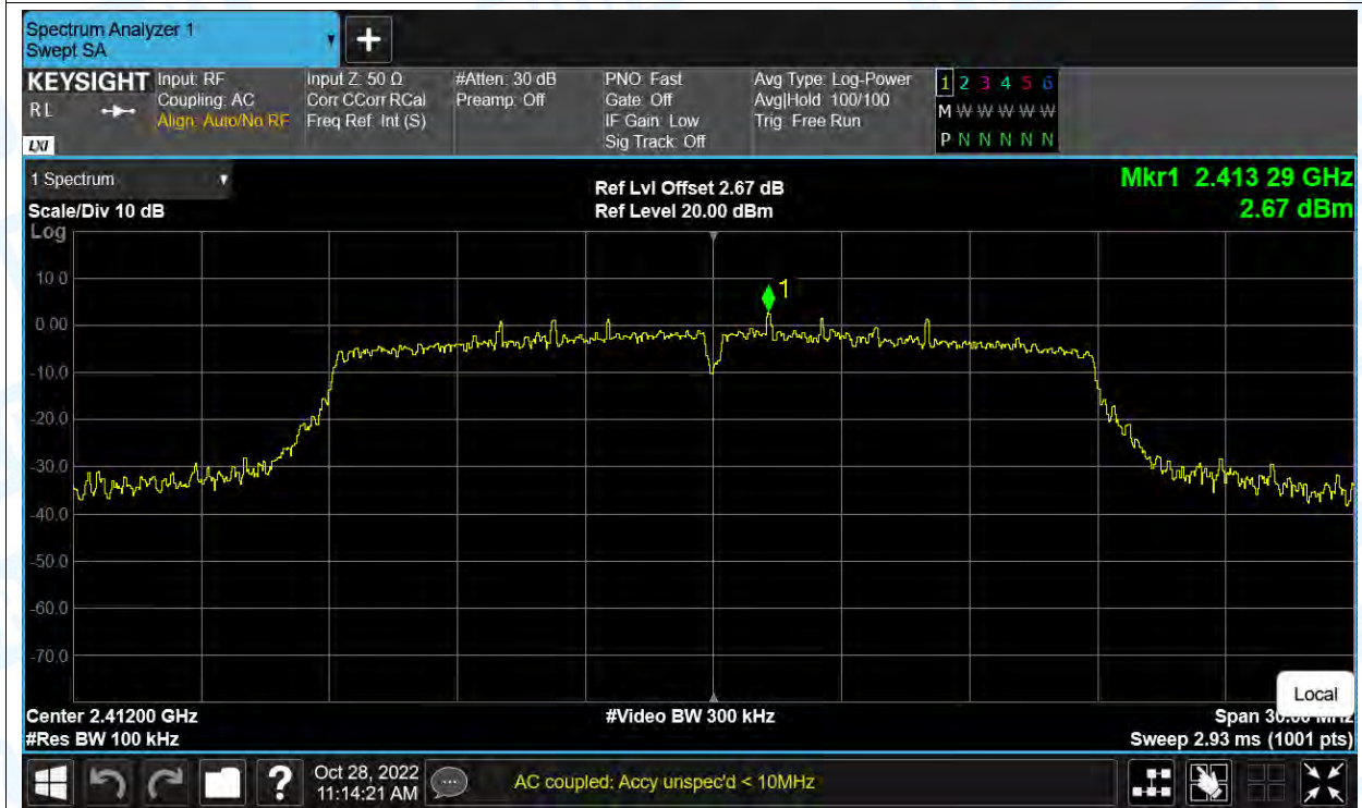
Band Edge NVNT g 2412MHz Ant1 Emission
