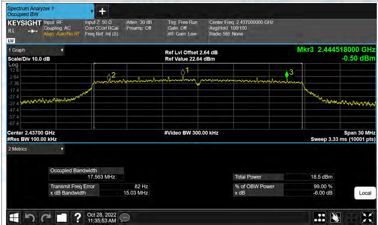
-6dB Bandwidth NVNT n(HT20) 2437MHz Ant1
