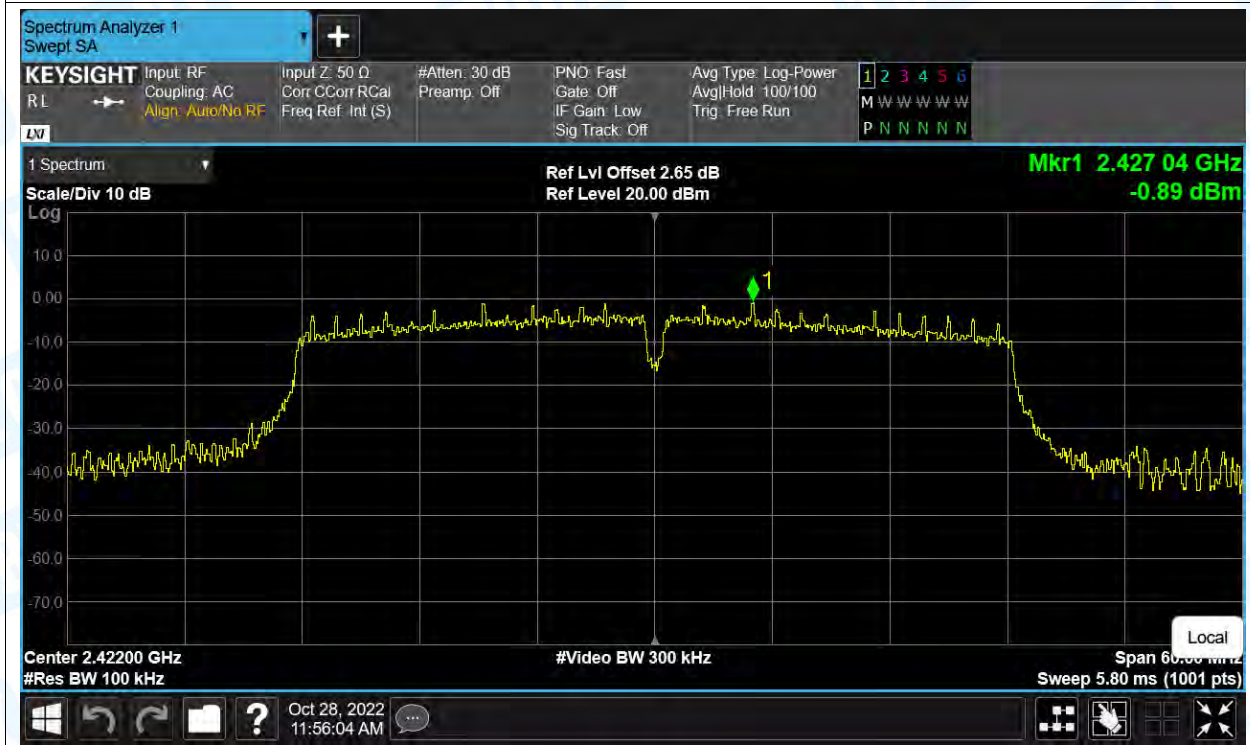
Tx. Spurious NVNT n(HT40) 2422MHz Ant1 Emission
