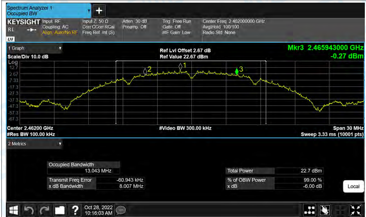
-6dB Bandwidth NVNT g 2412MHz Ant1
