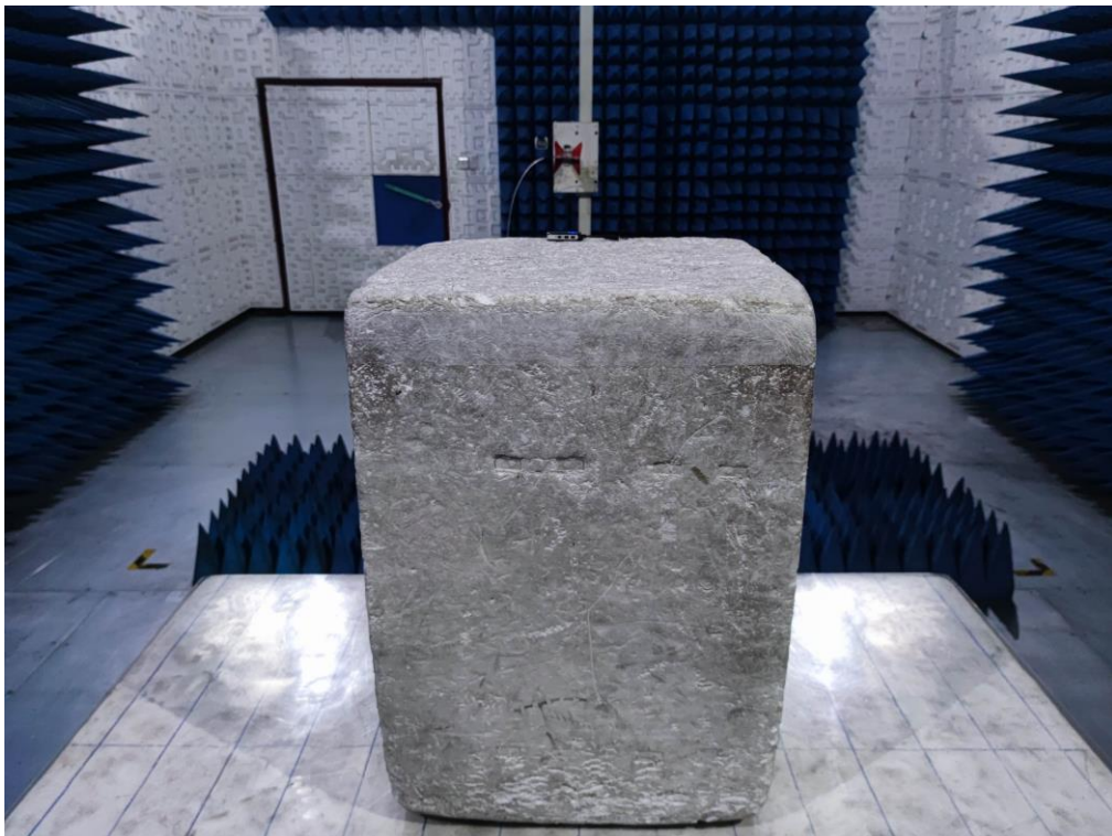
RADIATED EMISSION TEST SETUP ABOVE 1GHz
