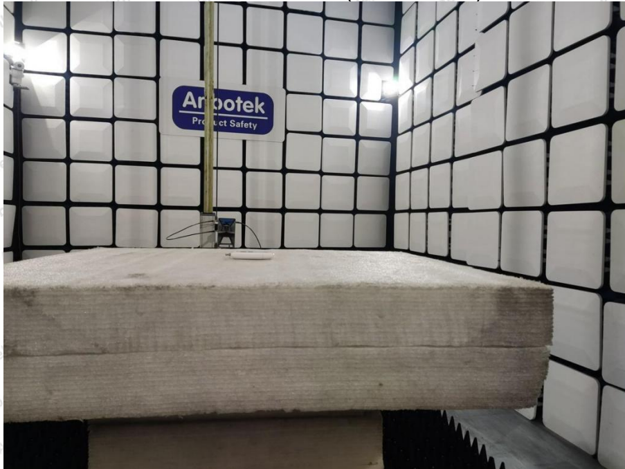
Radiated Emission (above 1GHz)
