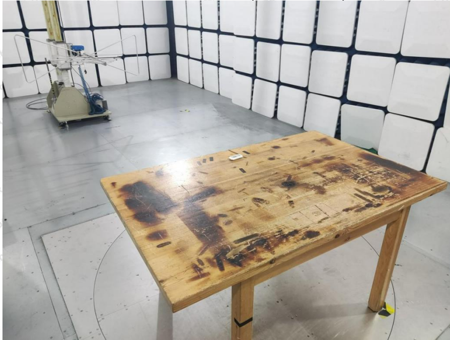
Radiated Emission (below 1GHz)
