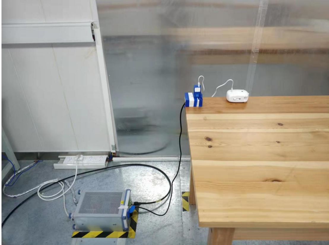
Conducted emission test setup
