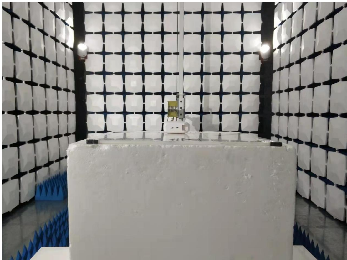
Above 1GHz for radiated emission test setup
