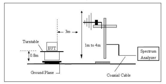
(C) Radiated Emission Test-Up Frequency Above 1GHz
