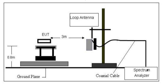
(B) Radiated Emission Test-Up Frequency 30MHz~1GHz
