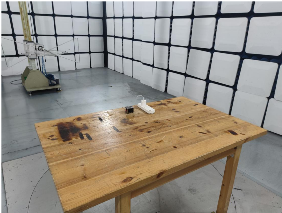
Photo of Radiation Emission Test
