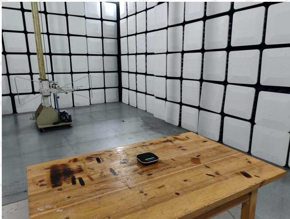
Photo of Radiation Emission Test
