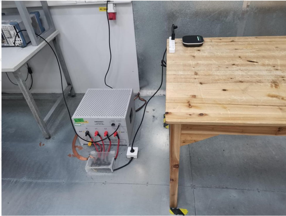
Photo of Conducted Emission Measurement
