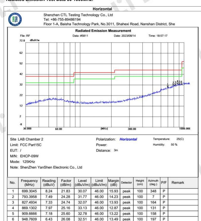
Radiated Emission Test Data 30-1000MHz:
