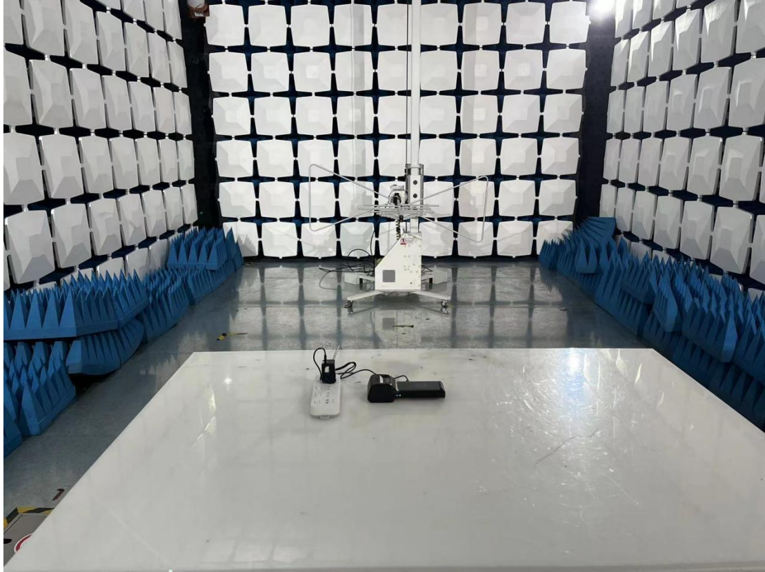
Above 1GHz for radiated emission test setup
