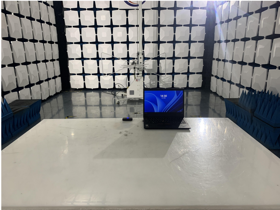
Above 1GHz for radiated emission test setup
