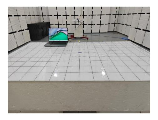
**Set-up for Radiated Spurious Emission, Above 1GHz**
