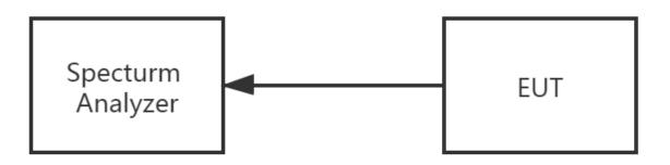
The EUT is connected to the Spectrum Analyzer; the RF load attached to the EUT antenna terminal is 500hm; the path loss as the factor is calibrated to correct the reading. Tune the measurement with the spectrum analyzer's resolution bandwidth (RBW) = 100 kHz. In order to make an accurate measurement, the span is set to be greater than RBW.
