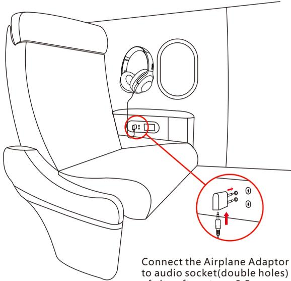
Connect the Airplane Adaptor to audio socket(double holes) of aircraft seat,use 3.5mm audio cable to connect with your headphone and Airplane Adaptor.
