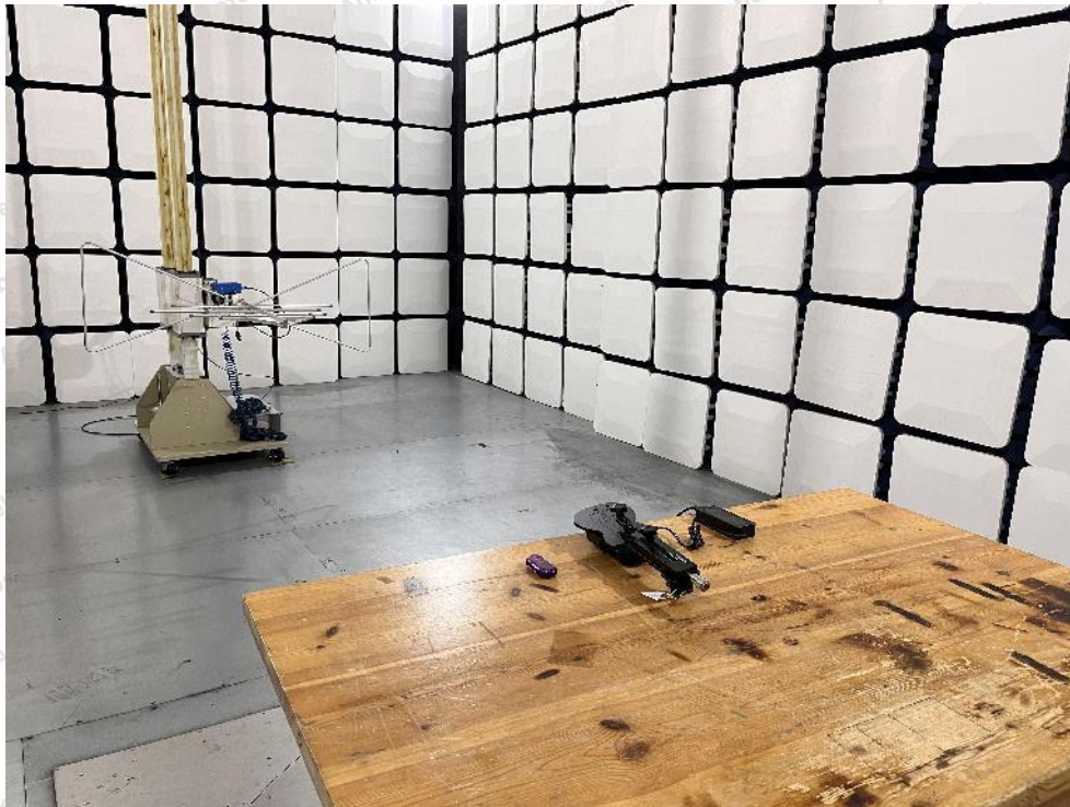
Photo of Radiation Emission Test
