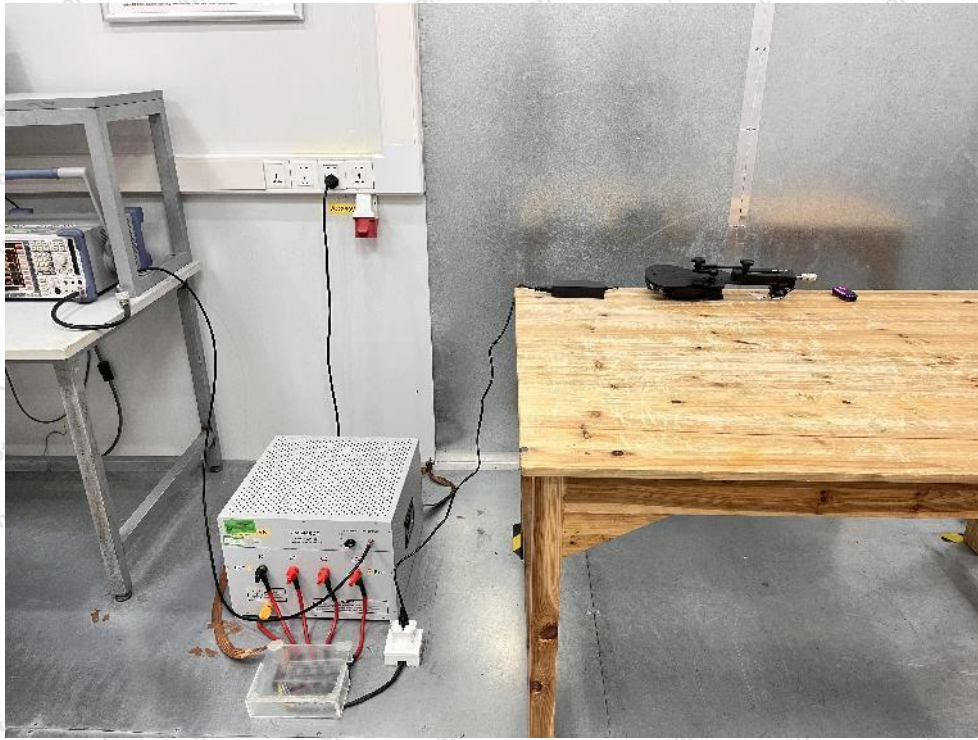
Photo of Conducted Emission Measurement
