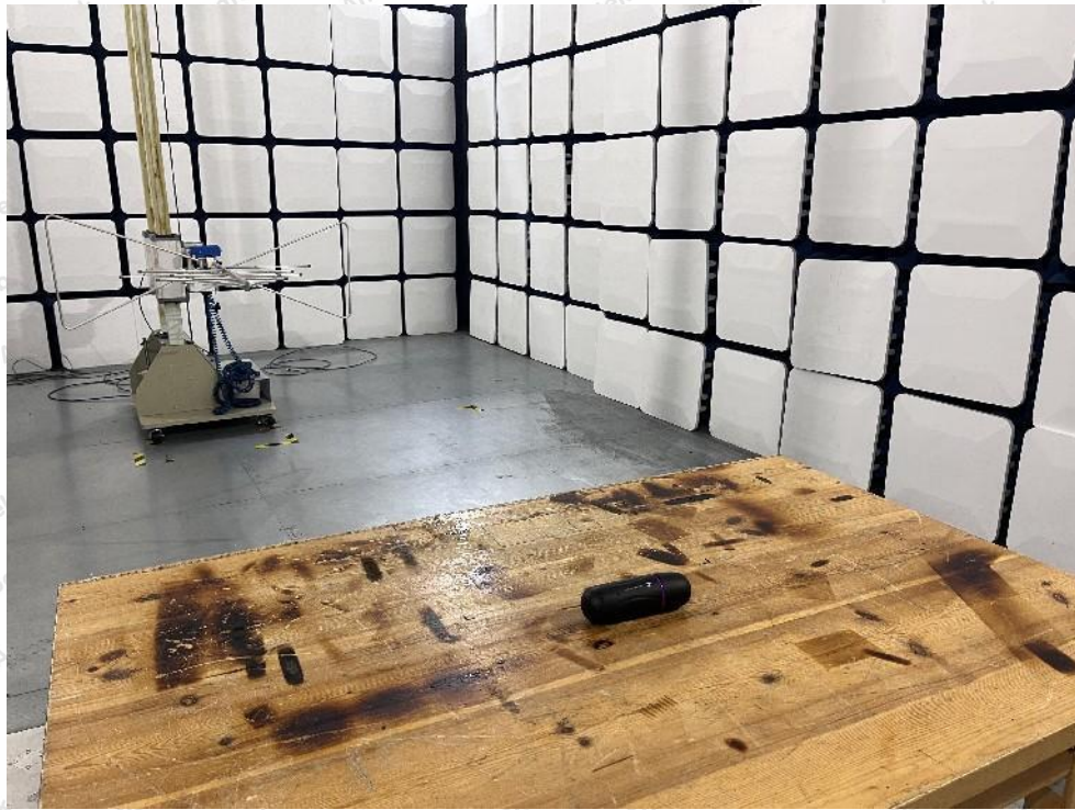
Photo of Radiation Emission Test
