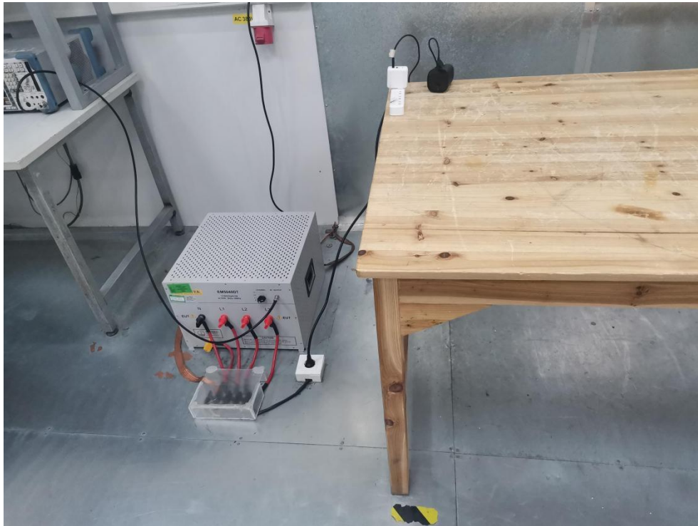
Photo of Conducted Emission Measurement
