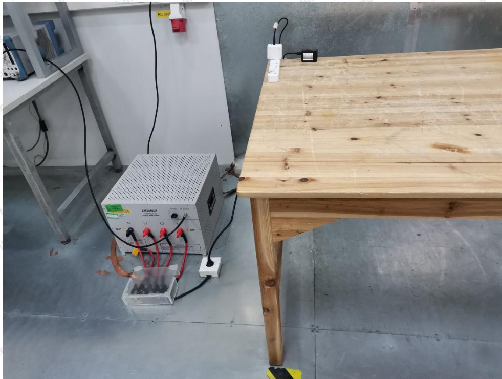
Photo of Conducted Emission Test
