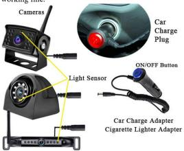
Use the cigarette lighter adapter to connect every camera with cigarette lighter socket (charge plug) in cab to turn on the camera, and use your finger to cover the light sensor of the camera to check if the infrared led lights turn red. If infrared led lights turn red, it means the camera is fine.
