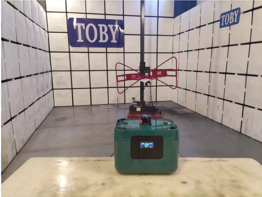
Photo of Setup for Radiated Emission (9KHz-30MHz)
