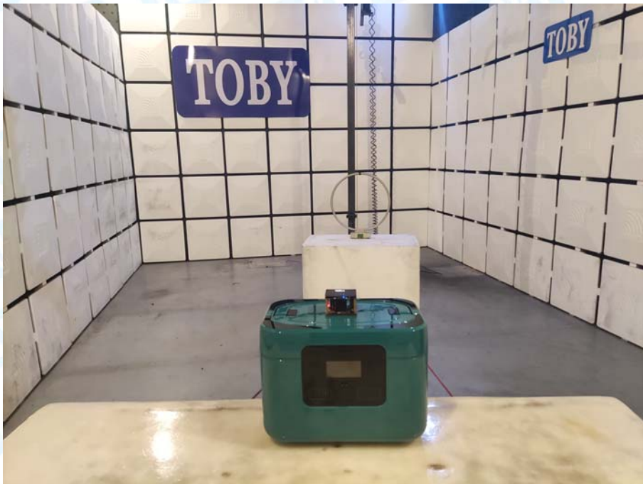
Photo of Setup for Radiated Emission (9KHz-30MHz)
