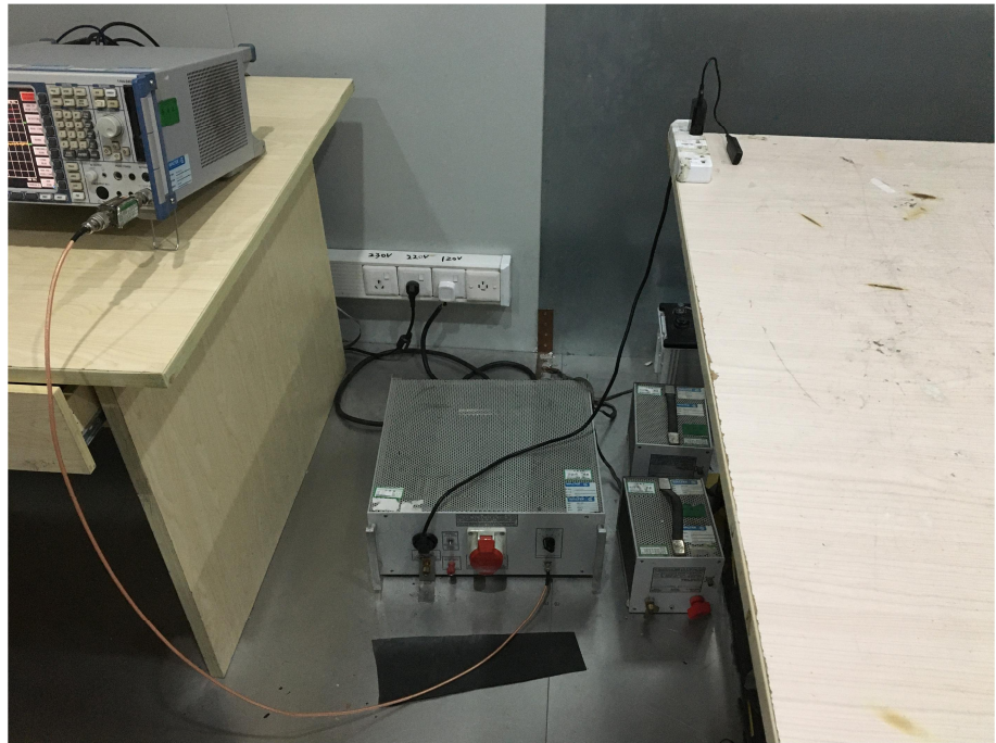
Conducted Emission Test Setup
