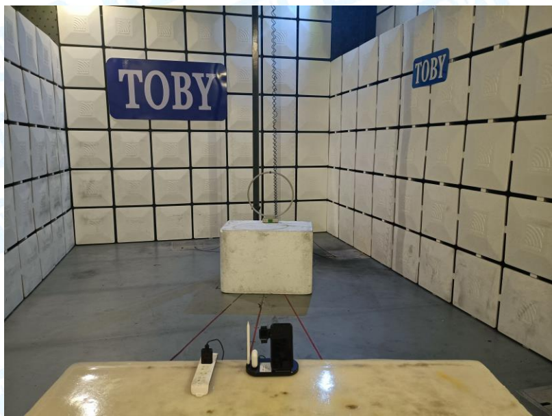
Photo of Setup for Radiated Emission (9KHz-30MHz)
