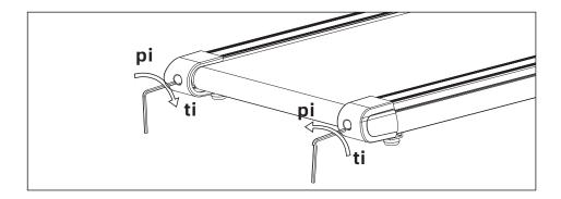
If the running belt is turned to the left: adjust the left bolt clockwise or the right bolt counter clockwise.
