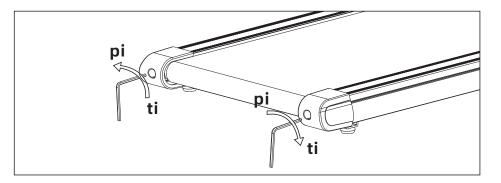
If the running belt is turned to the right:, adjust the right bolt clockwise or the left bolt counter clockwise.
