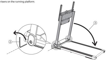
4. As shown in step ④: Lock the bolts under the left and right upright columns clockwise with an Allen wrench and fold them.
