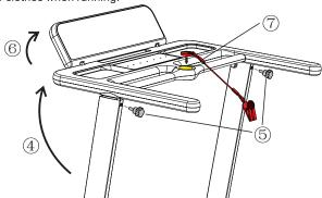
4. As shown in step (a) below, after the riser is locked, fasten the riser cover on the left and right risers respectively. Plug in the power cord, Step into the front socket, turn on the power, turn on the power switch below the front of the machine, and enter the standby state.
