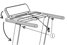
2. As shown in step ② of the figure: Loosen the bolts under the left and right upright columns by using an Allen wrench counterclockwise for 3 to 4 turns.
